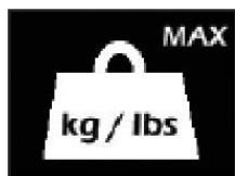
If the lift stops because of an overload (an attempt to lift more than the safe working load) the overload symbol will appear on the LCD display and the lift will cease to operate until the additional load (above the SWL) has been removed.
